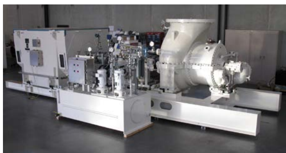
Figure 3. Modular Turbine-Generator Set Ready to Ship from Factory
