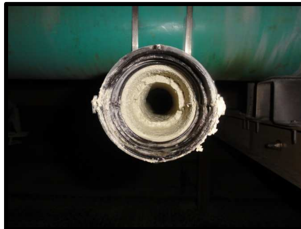
Figure 3: Sulphur deposits in a cooling water pipe.
