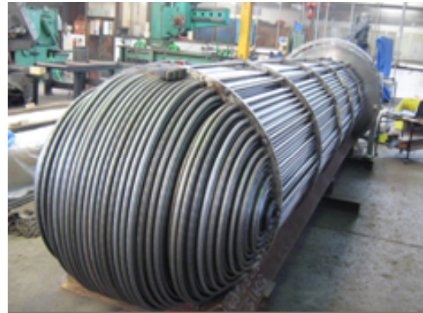
Figure 3 'U' Tubes Steam Generating Hex
