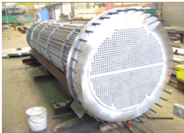
Figure 4 Tube Plate, Steam Generating Hex
