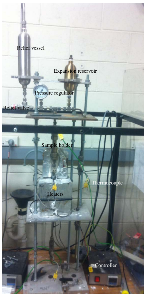
Figure 4: Flow-through cell used for rock-water interaction experiments.
