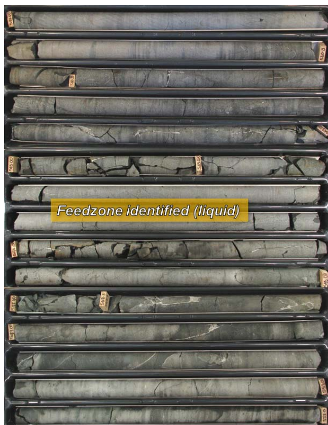
Appendix Figure A: Core photos from THM-18, showing feed zone in Spa Andesite
