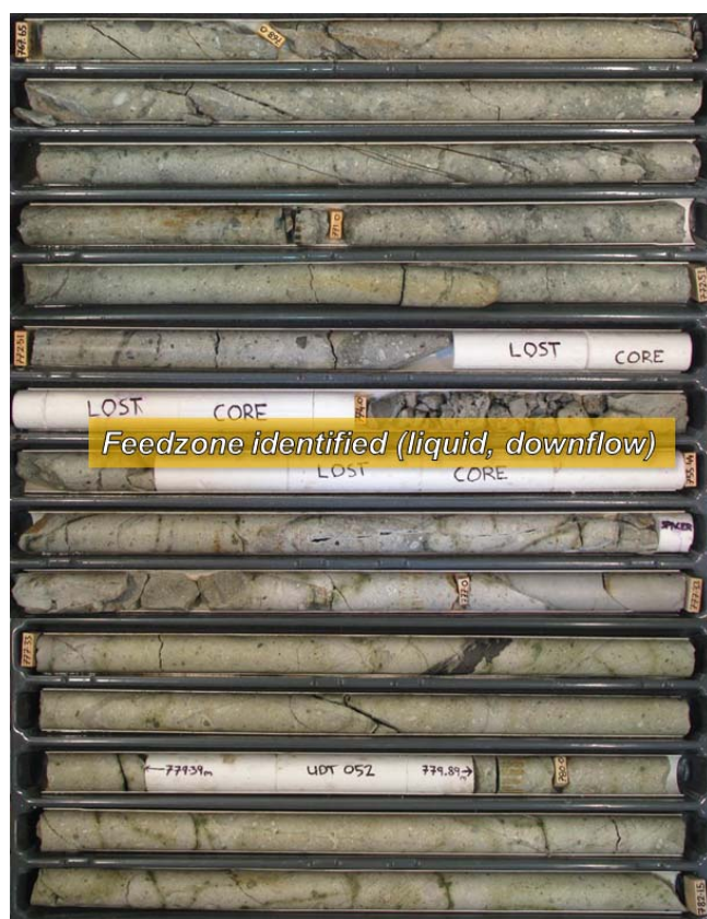
Appendix Figure A: Core photos from THM-18, showing feed zone in Spa Andesite
