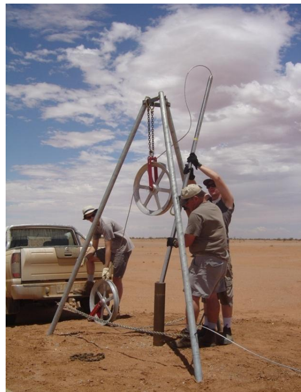
Figure 3: 15Hz Sensor Being Deployed Into The Paralana-1b Borehole. Station Name = B05
