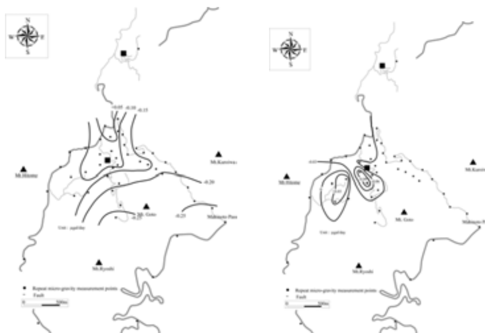
Fig.3: Gravity change at Hatchobaru geothermal field. Left: from June 1990 to June 1992, Right: from October 2000 to October 2001.
