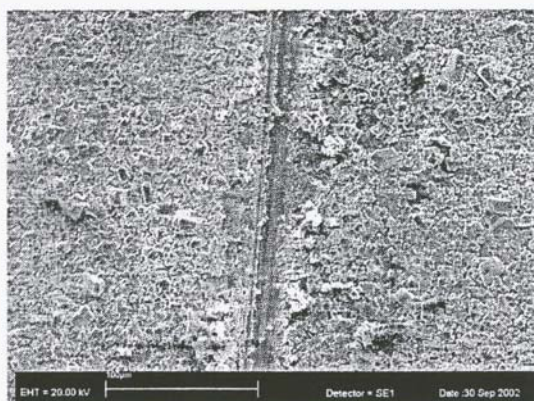
Figure 1: SEM View of Corrosion Product Scale on Carbon Steel, 150°C, 6 bar(a), pH 3 Adjusted to pH 5.
