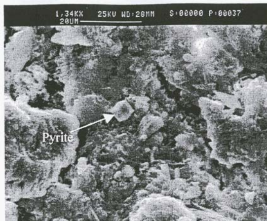
Fig. 5 Micrograph of the particulate matter in a filter from the Punta Mita water samples that shows a euhedral pyrite crystal.
