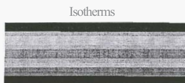
Figure 2. Porous medium heated from the top (50 °C) and cooled from below (20 °C), A=3 .
