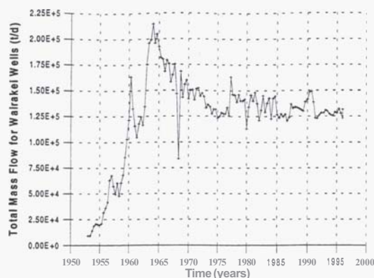
Figure 3 - Total Mass Flow from Wells at Wairakei
