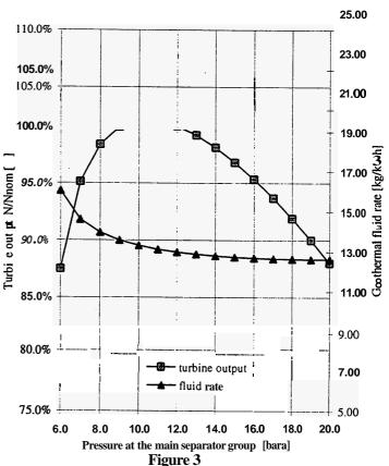
Medium Enthalpy Case: Effect of Separation Pressure on Turbine Output and Fluid Rate
