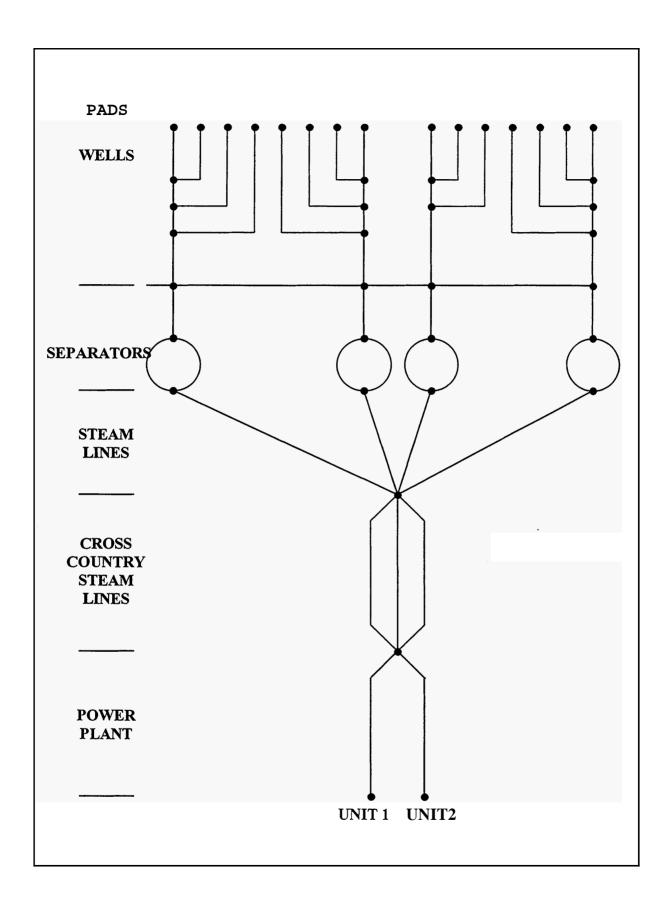
Figure 1 Steamfield Schematic
