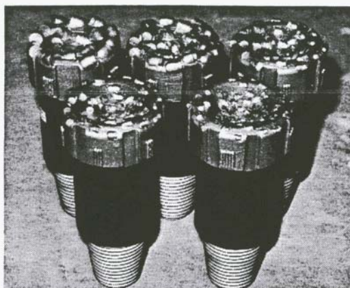
Figure 1- PDC full-face bits with 98.43mm diameter
