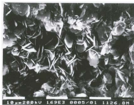
Figure 3a: Electromicrograph taken with SEM of illite in sample OK1:1126.8m.
