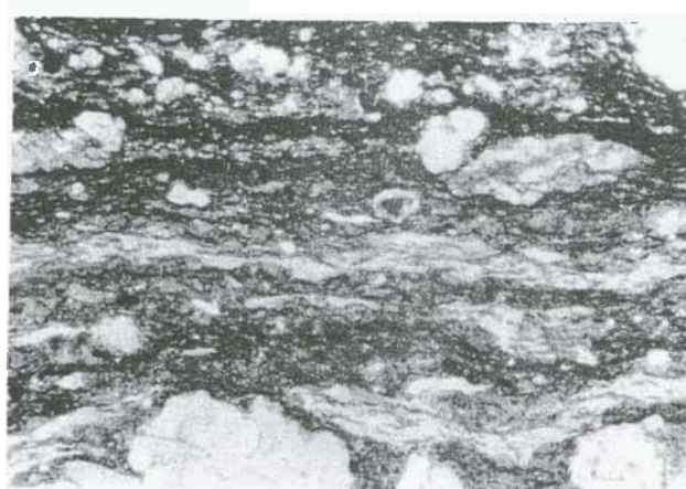
Plate 1. Attenuated lenses of chert formed due to compaction of the sediments (PPL). Field of view is 2mm.
