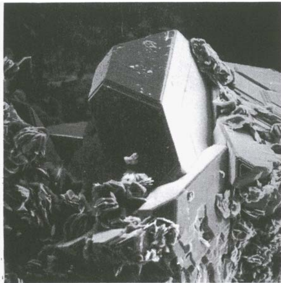
SPHALERITE AND CHLORITE GROWING INTO CAVITIES, B-16 CORE. Photo: B.G. Weissberg, DSIR.
