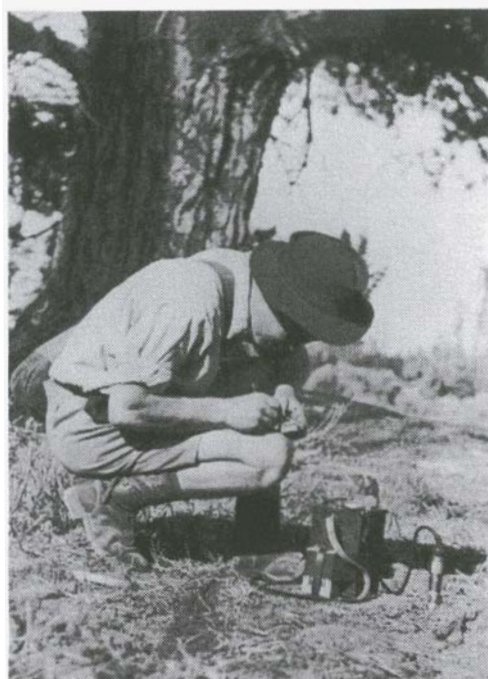
Gordon Dawson using Geiger counter on soil radioactivity survey, Wairakei to Taupo, late 1950
