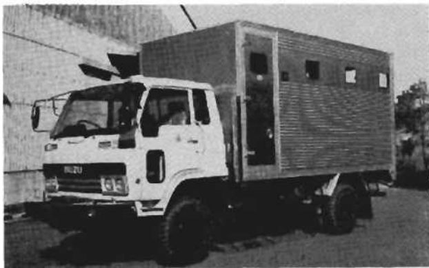
Photo. 1. Cable winch mounted 4-wheel drive truck.
