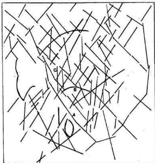
Fig. 7: Main faulting systems observed after processing of band 7 and DTM with the artificial illumination technique. A) Mastaloya fault, B) Las Papas fault and C) Los Humeros fault.
