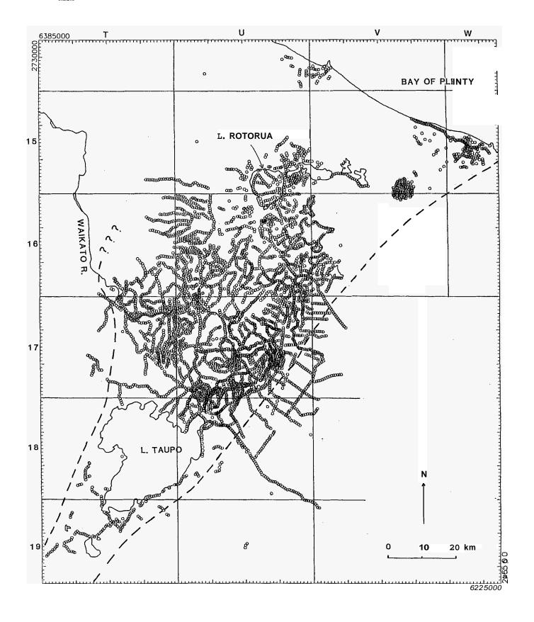
Fig. 1: Locations of resistivity measurements made between 1963 and January 1985 as part of the reconnaissance resistivity mapping project using either Wenner array (with spacing a = 550 m) or Schlumberger array (with spacing AB/2 = 500 m). Lettering at the edge of the map refers to the New Zealand Map Grid coordinates (in metres) and map sheet labels. Dashed lines indicate the approximate limits of the Central Volcanic Region.
