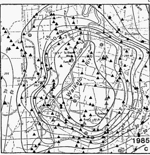
Fig. 2: Reconnaissance resistivity surveys of the Broadlands/Ohaaki geothermal field. All values shown are resistivities in ohm m.
