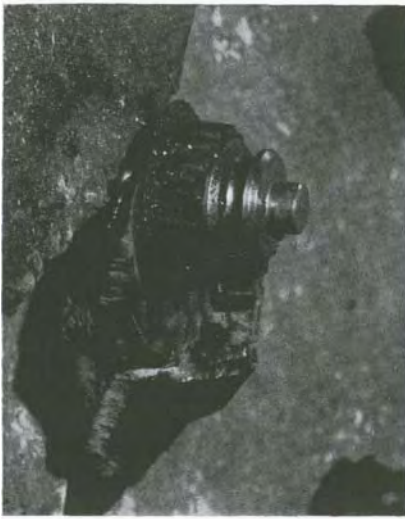
Fig. 8 Cast-iron cuttings entered into the roller bearing.
