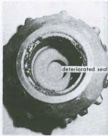
Fig. 9 The elastmer seal broken by thermal deterioration.
