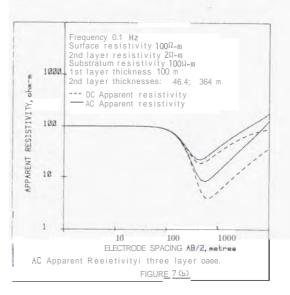
For AB/2  $\lesssim$  800 m the form of the curves is that of a normal descending type of sounding curve. Standard layer <code>mode1</code> interpretation of the initial part of the curves implies that resistivities of less than  $10^{\Omega}$ -m occur throughout the survey area.
