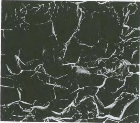
Fig. 5 Predominantly intergranular fracture: stress, 366 MPa endurance, 8.4 \times 10^5 cycles. x 1000 mag.
