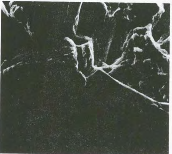
Fig. 7 Oblique metallographic section through C.F. fracture, showing two phase structure of ferrite and martensite. x 1500 mag.
