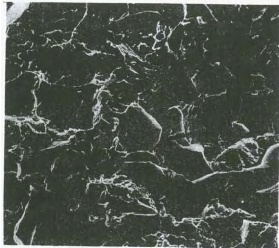
Fig. 6 Transition of corrosion fatigue crack (bottom right) to brittle fracture (top left). x 1000 mag.
