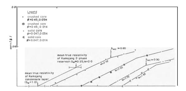
Figure 1: RESISTIVITY OF SATURATED AND PARILY SATURATED CRUSHED ROCKS AND CORES (RHYOLITE).
