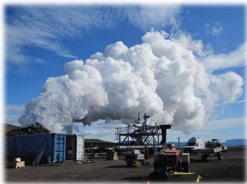
Fig. 2. The flow of the IDDP-01 into a rock muffler produced dry superheated steam with only 0.1-0.2% of non-condensable gases. (Photograph courtesy of Kristján Einarsson).
