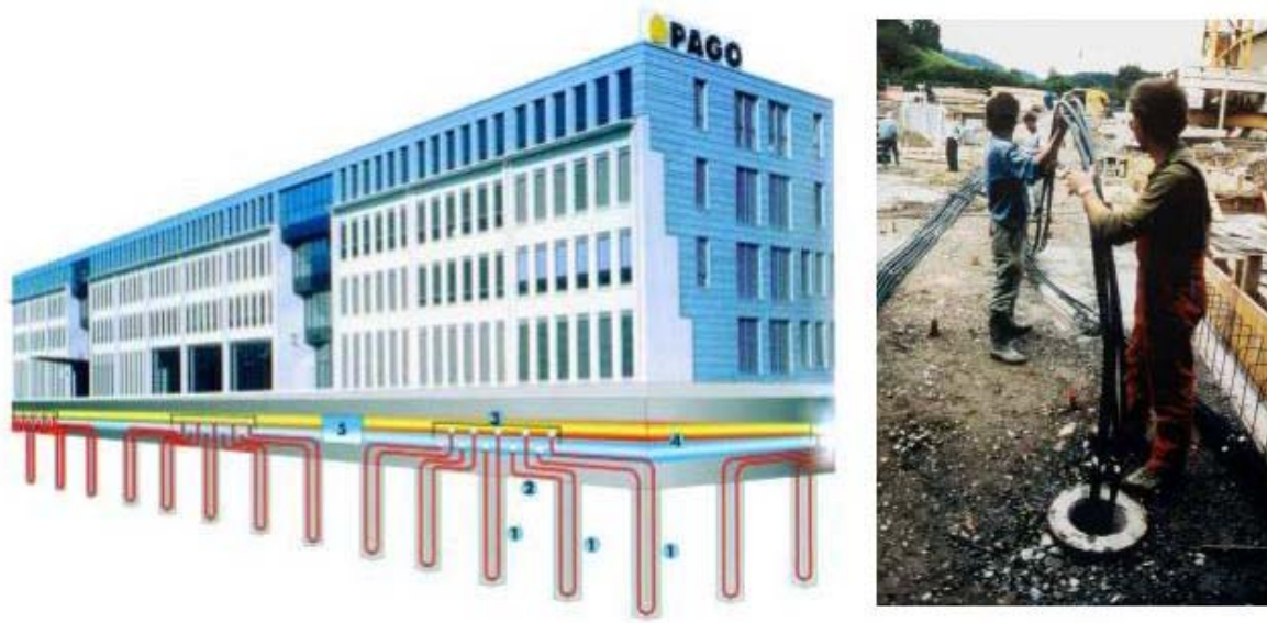
Fig. 2 Sketch of energy piles below buildings (left), installation of heat exchanger loops in piles (right).
