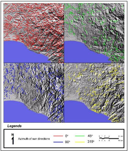
Figure 6. Results of lineaments delineation method from four different illumination directions, i.e. 0°, 45°, 90°, 315°.
