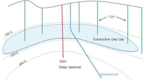
Figure 2: Generic drilling options (TGH = temperature gradient hole, DSH = deep slimhole)
