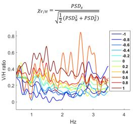
Figure 7: Result of the V/H spectral curves classification
