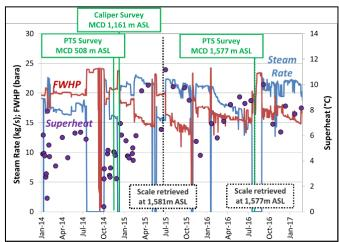
Figure 7: Historical steam rate, FWHP, superheat, and Maximum Clear Depth (MCD) at DRJ-AC during 2014-2017.
