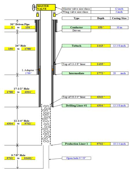
Figure 3: Well completion schematic of AWI 9-9
