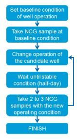
Figure 1. NCG Interference Test Workflow
