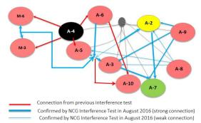
Figure 4 Salak NCG Interference Connectivity
