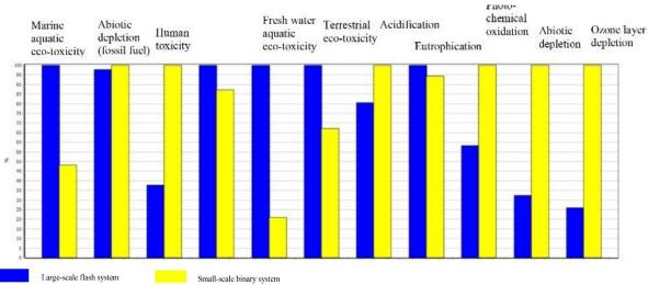
Figure 5 The LCIA of deep well drilling for the large-scale flash system and the small-scale binary system
