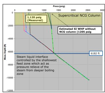
Figure 10: Shut-in PT survey of Awi 9-9. Presence of supercritical NCG column protecting the wellhead from exposure to higher pressure and temperature.
