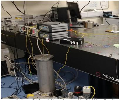
Figure 2: Experiment set up. (1) Laser, (2a) 2m red fibre under test cable, (2b) 100m yellow fibre under test fibre, (3) circulator, (4) Series of splitters, (5) cryogenic refrigerator, with SNSPD temperature sensor inside, (5) Hydraharp, (6) Measured liquid.
