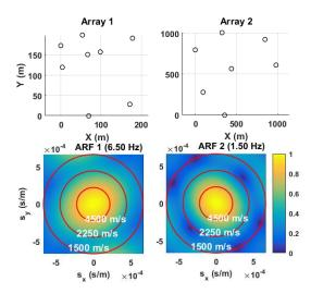
Figure 10: Geometry of the two arrays (top) and their response functions at the relevant frequencies (bottom)
