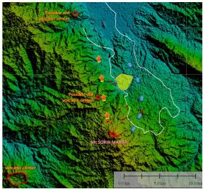
Figure 5: Interpreted outflow path from Mt. Sorik Marapi Upflow Zone to Sampuraga
