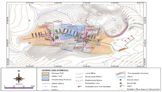
Figure 7. Geological Engineering Map at Landslide Area showing dominantly Orange Tuff at Awi-14
