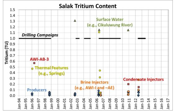
Figure 8: Historical tritium content at producers, brine injectores, condensate injectors, and surface water of Salak geothermal field.
