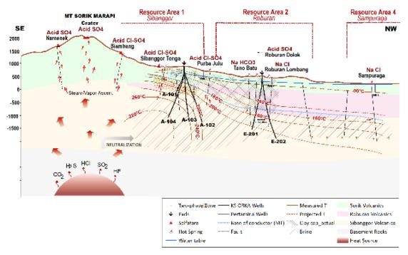
Figure 4: Updated Conceptual Model of the Sorik Marapi Geothermal Project
