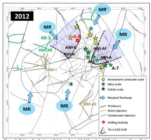
Figure 9: Tritium distribution at Salak geothermal field based on 2012 tritium sampling colletion (Modified from Syaffitri and Molling, 2013).
