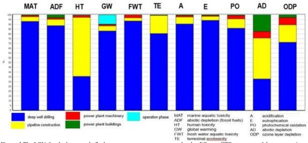
Figure 3 The LCIA for the large-scale flash system - percentage category for the different GTE processes of the construction, operation and disposal phases.
