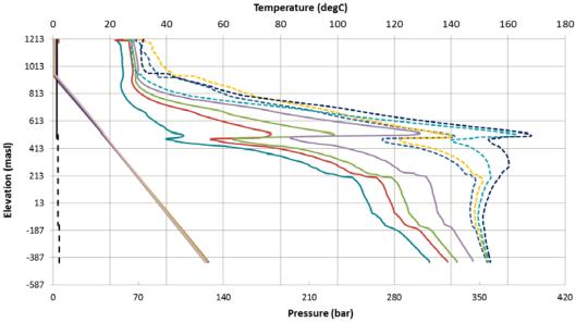
Figure 12: Anomaly in temperature recovery behind casing observed on E1 well that could be attributed to shallow steam
