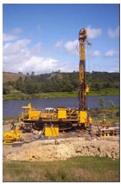
Figure 5: Typical slimhole coring rig
