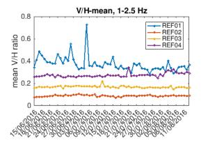
Figure 8: Mean V/H ratio evolution in [1-2.5] Hz over a two-months recording period
