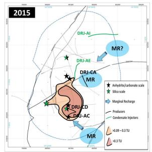
Figure 5: Tritium distribution at Darajat geothermal field based on 2015 tritium sampling colletion (Modified from Syaffitri et al., 2016).
