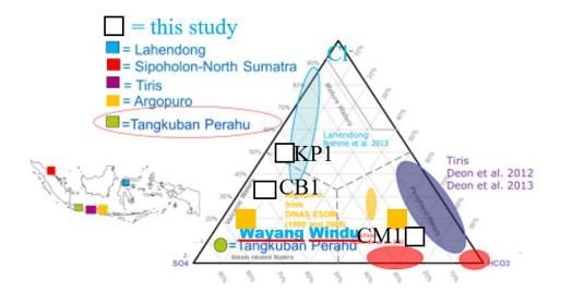
Figure 6: Ternary diagram of the major anions Cl<sup>-</sup>, SO<sub>4</sub><sup>2-</sup>, HCO<sub>3</sub><sup>-</sup>. Data from the literature show significant differences in the geochemistry from different fields and are included for comparison.
