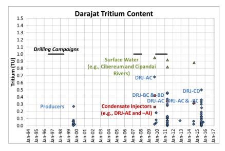
Figure 4: Historical tritium content at producers, condensate injectors, and surface water of Darajat geothermal field.
