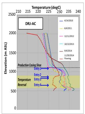
Figure 6: Historical PT profiles of DRJ-AC shows temperature reversal at 584 - 932 m ASL.
