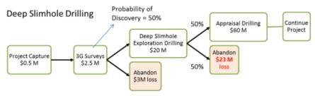
Figure 8: There is potential to exit a project at each major phase if the project does not prove viable. If Probability of Discovery from exploration drilling is low, then the use of deep slimholes puts less capital at risk than when using conventional wells for the exploration phase.
