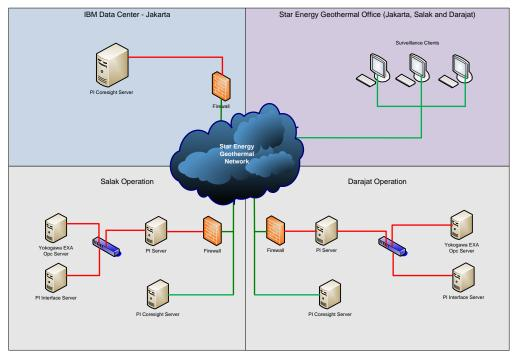
Figure 3. Surveillance system and data architecture flow diagram
