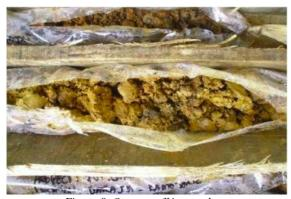
Figure 8. Orange tuff in core box
