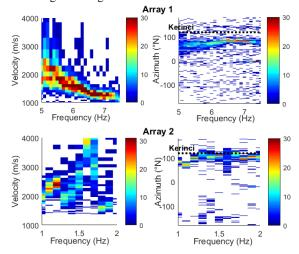
Figure 11: MUSIC: velocity-frequency and back-azimuth histograms over analyzed windows
