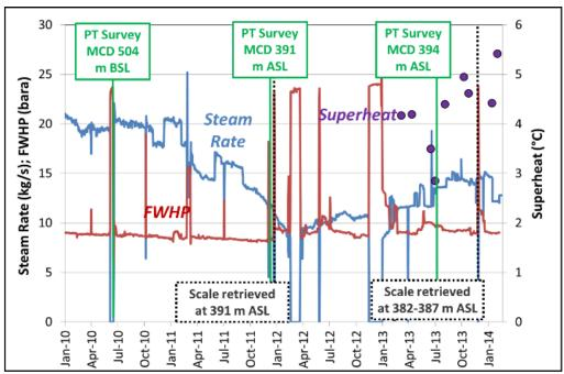
Figure 10: Historical steam rate, FWHP, superheat, and MCD at AWI-A-7 during 2010-2014.
