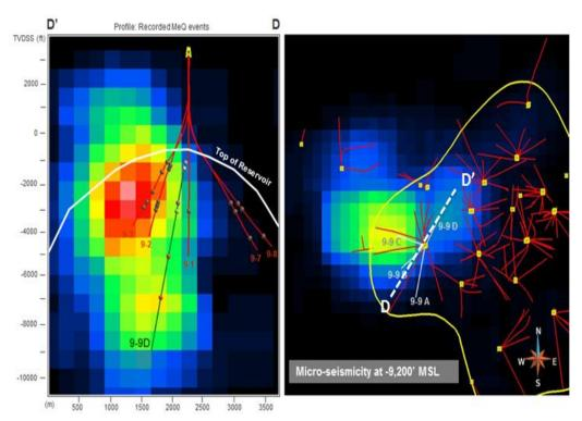
Figure 12: Recorded MeQ event at pad AWI 9 due to injected fluid movement in the deep reservoir. The map shows cumulative MeQ events from 1998 until 2014.
