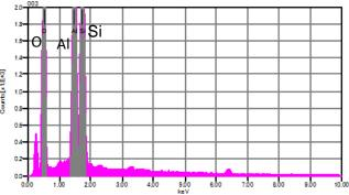
Figure 4: a) EMP image aquired on a plagioclase crystal where **the alteration patterns** are clearly visible in the plagioclase grain (left). b) EBS sprectum aquired on the alteration rims showing **kaolinite** occurrence (right).
