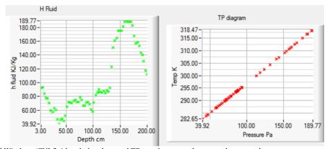
Figure 9: LabWindows/CVI fluid enthalpy data and TP graph output of measured saturated water temperature along 2m fibre under test.
