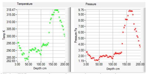
Figure 8: LabWindows/CVI Temperature and pressure data output of measured saturated water temperature along 2m fibre under test.
