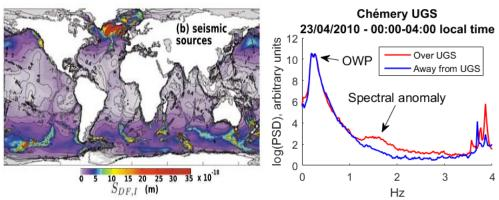
Figure 1: Source zones of seismic ambient noise (after Ardhuin et al., 2011) - Typical spectra of seismic signals outside (blue) and over (red) an Underground Gas Storage
