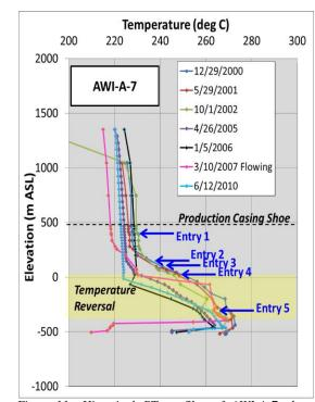
Figure 11: Historical PT profiles of AWI-A-7 shows temperature reversal at 19 - 465 m BSL.
