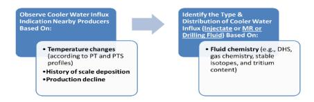
Figure 3: Flowchart to investigate the cooler water influx type and its distribution at Darajat and Salak geothermal fields.
