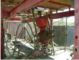
Figure 6: Blowout Preventer for slanted slimhole drilling
