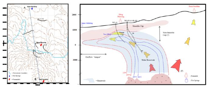
Figure 4: North-south cross section showing conceptual model of Muara Laboh field (Situmorang et al., 2016)
