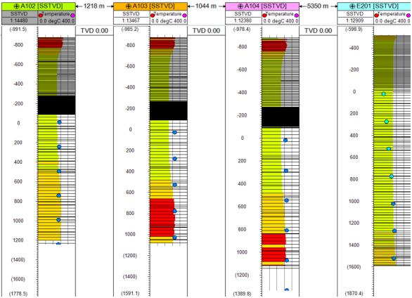
Figure 18: Well section window to compare original well data temperature (blue circle symbol) and result model of temperature
