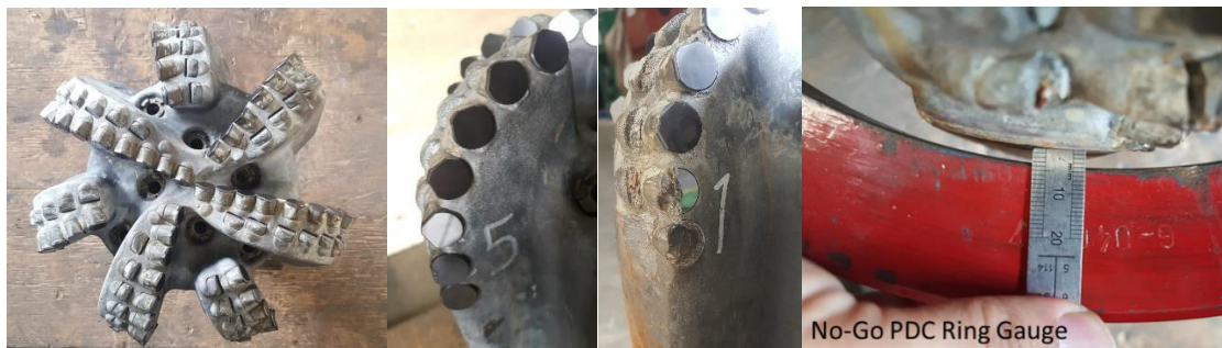
Figure 6: The dull condition of the 12 ¼" PDC bit used on subject well. Most cutters were still in good condition. Some cutter on the gauge was damaged. The bit was undergauged 3/16".
