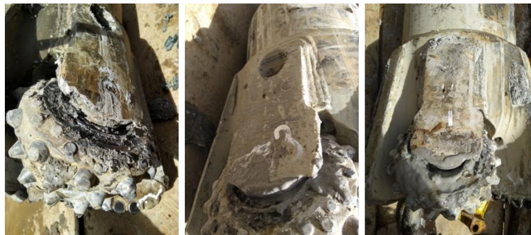
Figure 5: Condition of leg and shirrtail after run in Well T7.
