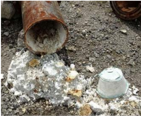
Figure 2. Silica Scaling at Dieng field ( Felix Arie Setiawan, 2015)
