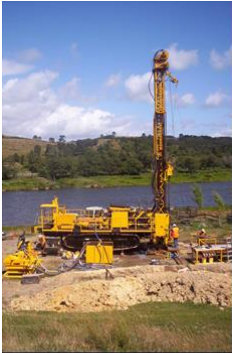
Figure 5: Typical slimhole coring rig
