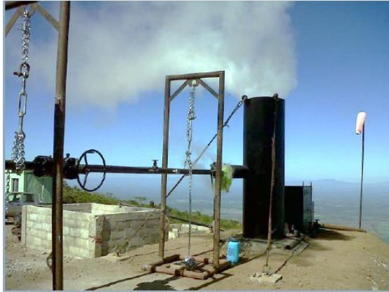
Figure 13: Slimhole well CSS-01 on discharge; note that the water vapour is coming out the silencer with none coming from the weir box indicative of a dry discharge.
