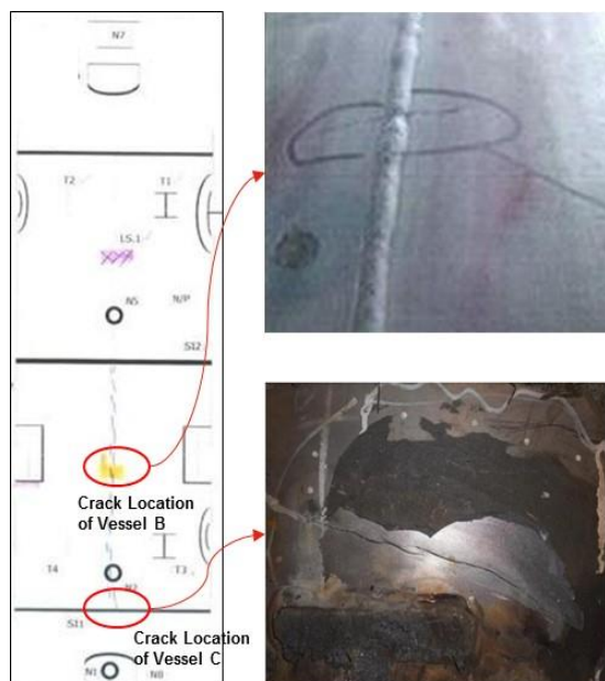
Figure 2 Crack and origin location for both examined samples.
