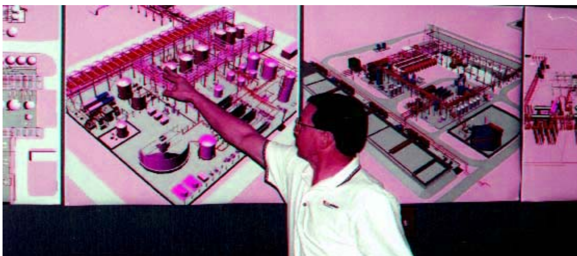
Figure 1: CalEnergy engineer pointing out the minerals recovery facility, with the ion exchange and solvent extraction plant on the right and the electrowinning facility on the left (Clutter, 2000).
