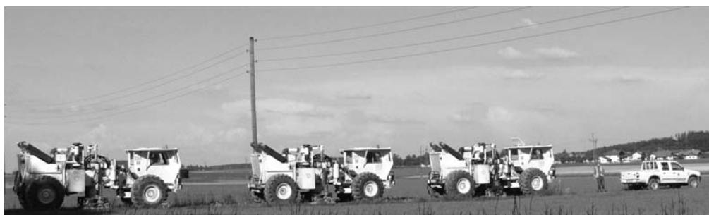
Figure 7: Vibrators of Deutsche Montan Technologie (DMT) used for the seismic survey.
