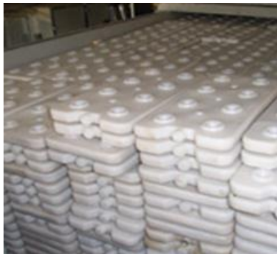
Figure 7: PCM encapsulated in rectangular plastic containers [PCM Products Ltd, 2011].
