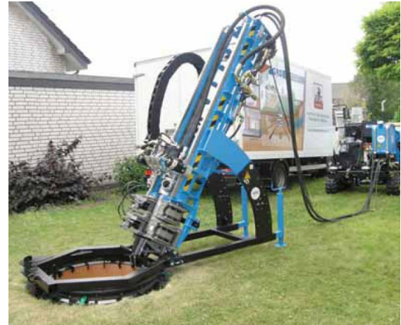
Figure 5. GRD-drill rig from Tracto-Technik, remotely controlled during transport (left) and ready for drilling, with drill rig detached from motor unit and positioned separately (right) (photos Tracto-Technik GmbH & Co. KG)
