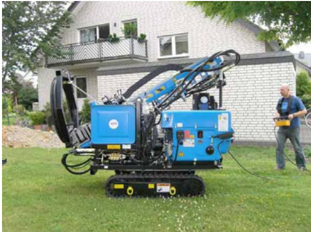
Figure 5. GRD-drill rig from Tracto-Technik, remotely controlled during transport (left) and ready for drilling, with drill rig detached from motor unit and positioned separately (right) (photos Tracto-Technik GmbH & Co. KG)
