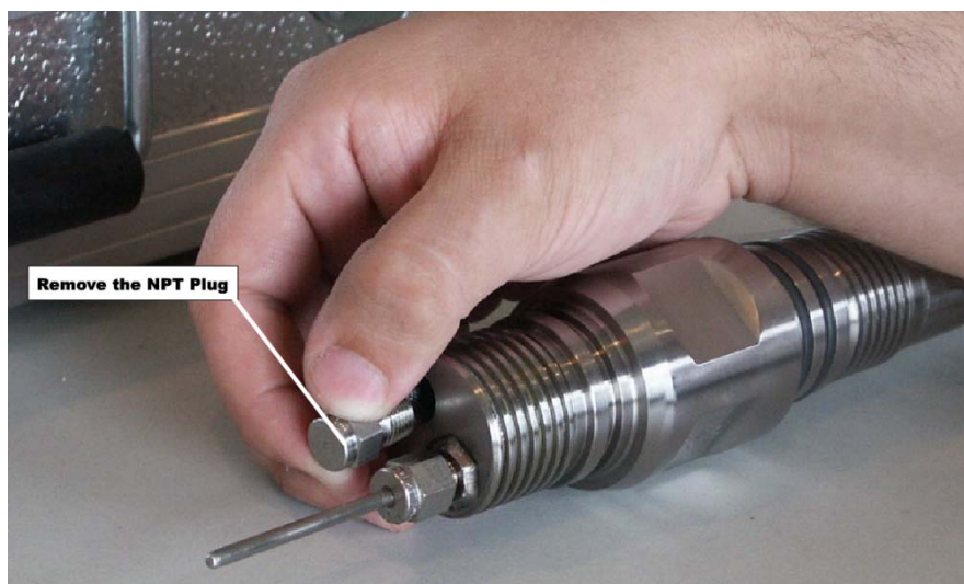
Figure 2: External platinum temperature sensor and capillary opening (NPT plug) for pressure readings.
