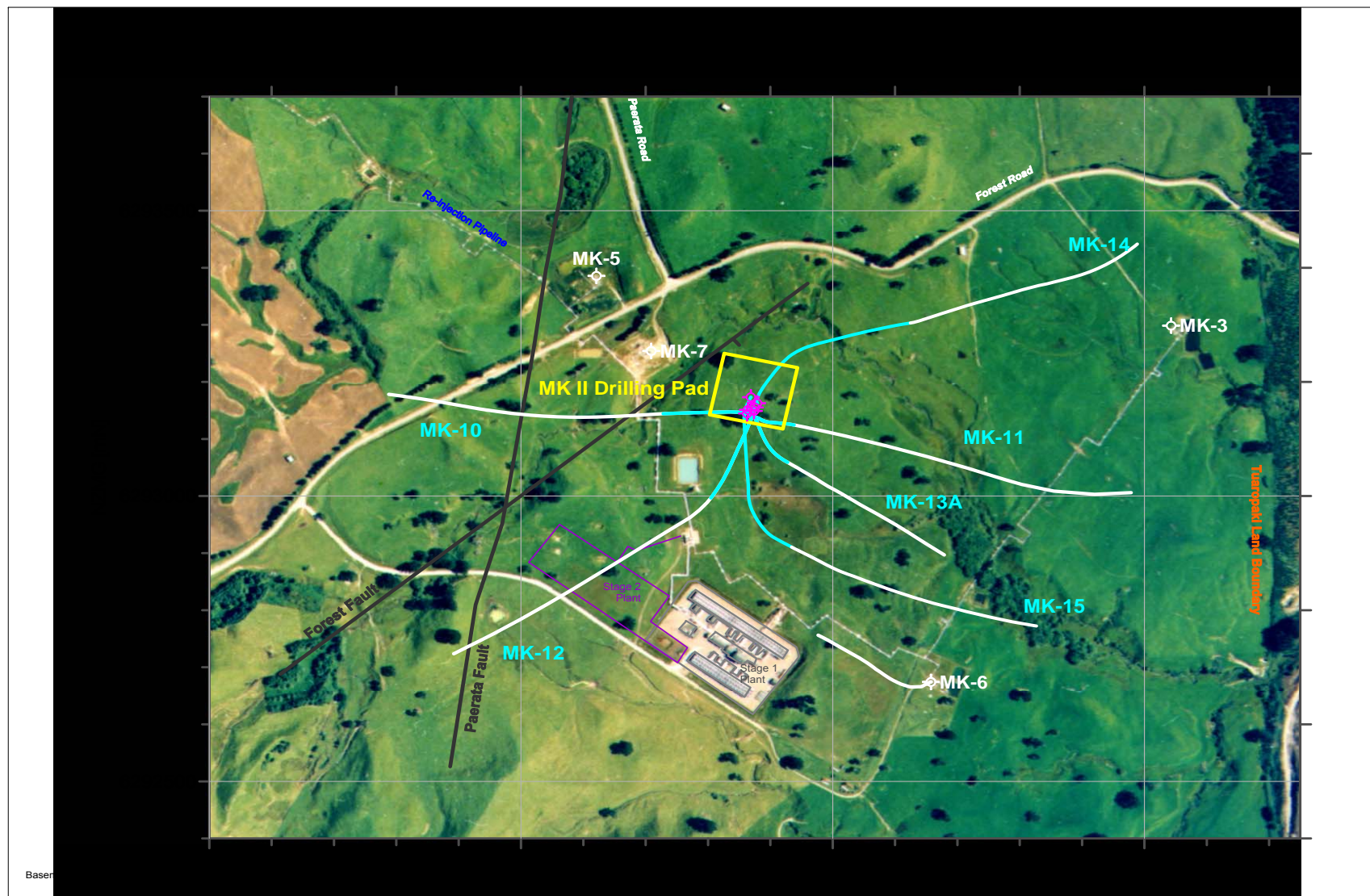
Figure 10. Mokai, Well Pad MK-II with Wells MK-10, MK-11, MK-12, MK-13, MK-14 and MK-15 as drilled Well Tracks (Cased sections indicated in grey/green; Production sections indicated in white).
