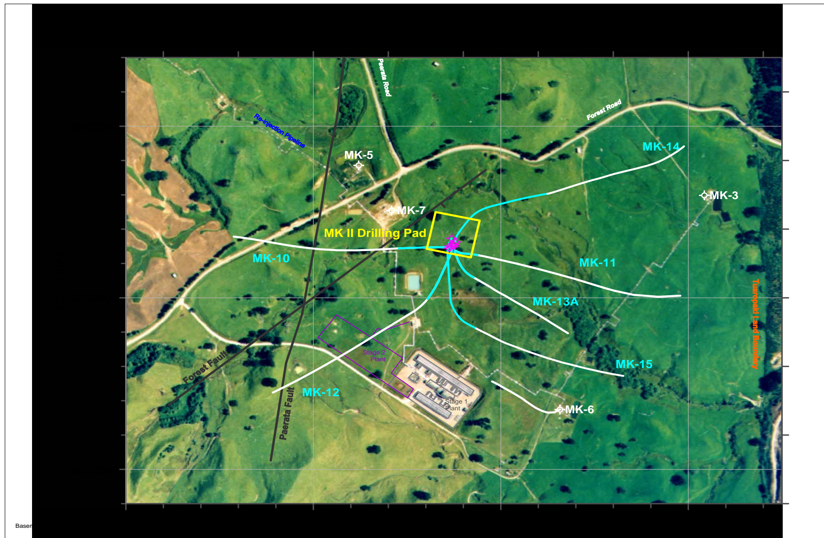
Figure 10. Mokai, Well Pad MK-II with Wells MK-10, MK-11, MK-12, MK-13, MK-14 and MK-15 as drilled Well Tracks (Cased sections indicated in grey/green; Production sections indicated in white).
