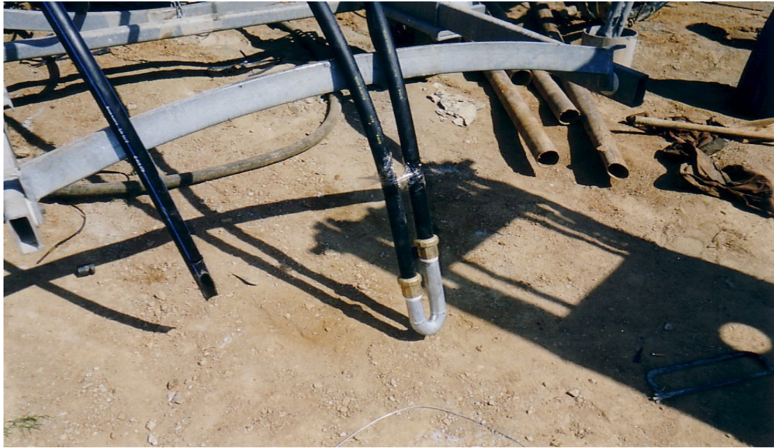
Photo 2: A VEHE and the U-Tube configuration.
