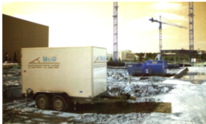
Figure 12: Schematic of Thermal Response Test and the equipment on site
