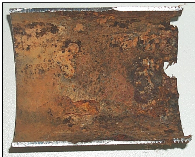
Figure 4. Picture of a corroded geothermal iron pipe section in contact a bronze valve.
