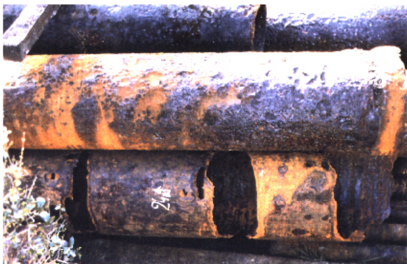
Figure 3: Underdeposit corrosion in carbon steel pipes from the Villeneuve La Garenne (France) production well
