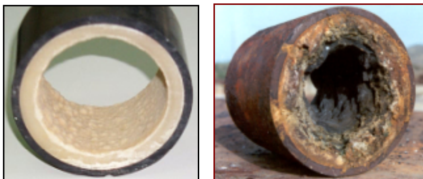
Figure 1. Pictures of scaled geothermal pipes. Left, \text{CaCO}_3 scales in a pipe carrying low-enthalpy geothermal water at Nigrita, Greece. Right, mixed silica and sulphide scales in the reinjection pipe of Milos geothermal plant.
