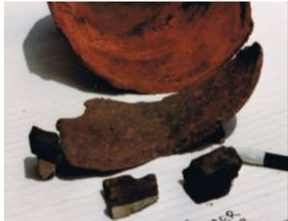
Figure 4: Corroded 8-5/8" casing recovered from BR25, 1983. In foreground is corroded casing (dark color) attached to cement grout (light color)
