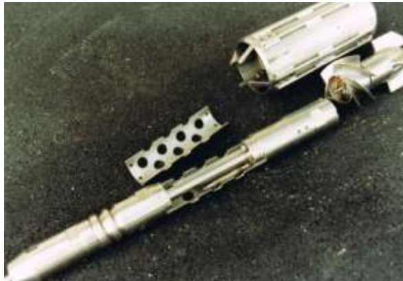
Figure 2: 1978 temperature-spinner instrument – no downhole electronics
