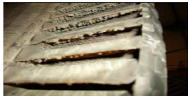
Figure 2: Stage 1 blade scaling Gunung Salak 55 MW turbine. Ref: Adiprana (2010)
