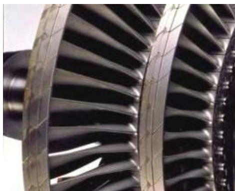
Figure 11: Integral covers with Z lock feature at the blade tip
