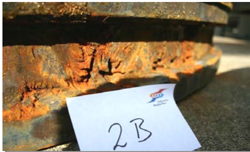
Figure 10: Outer Ring of carbon steel diaphragm with extreme water cutting erosion
