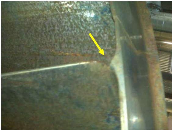
Figure 8: Blade tip erosion on an integral covered reaction blade
