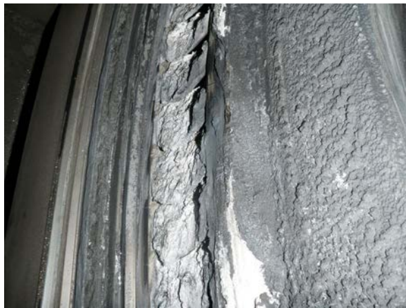
Figure 3: Stage 1 blade scaling on impulse steam turbine in geothermal service
