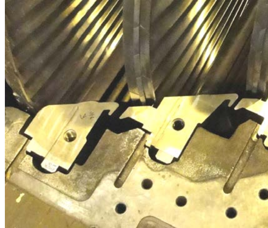
Figure 9: Moisture separators on an impulse geothermal steam turbine
