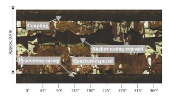
Figure 2. Coupling rupture as a result of quenching of IDDP-1 at approximately 300 m depth (Kaldal, et al., 2016).
