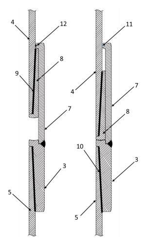
Figure 3. Concept drawing revealing the main principles of the flexible couplings. On the left is the coupling shown in open mode, on the right in closed mode. As shown the casing segment nr. 4 slides downward during warm up together with a sled nr. 8 and at given distance the coupling close by pressing the sled nr. 8 into a seat in the coupling lower part nr. 3. (Patent application no. 050129 – Thorbiornsson 2015).
