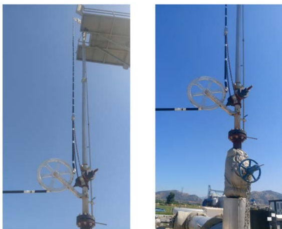
Figure 1: Wellhead fitted with lubricator assembly to allow installation of 6.35mm capillary tubing.
