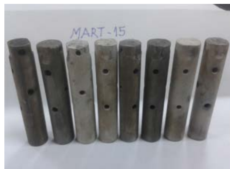
Figure 7: Retractable coupon from an injection well confirm effective metal silicate scale control.
