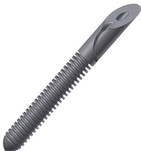
Figure 3: Pressure retention valve body with spiralled channel applied along a cylindrical cone.
