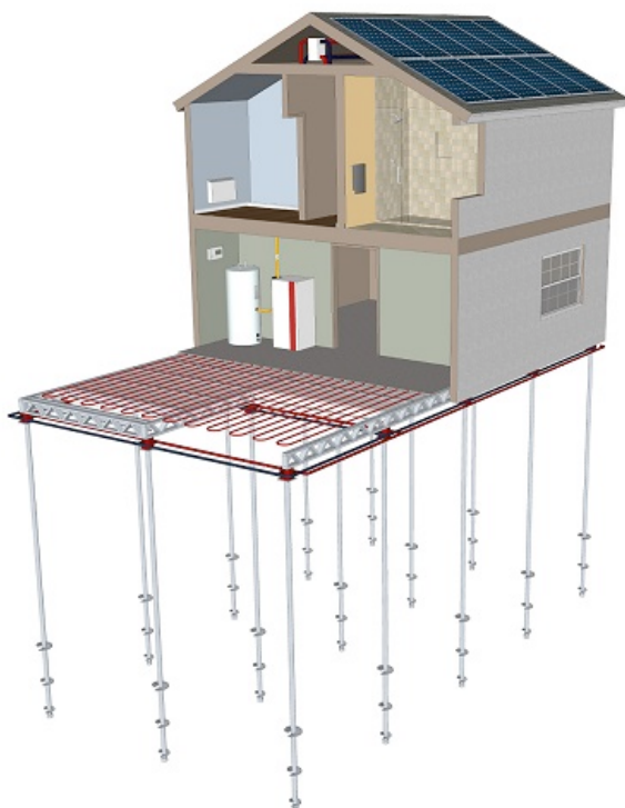
Figure 4: TSPs serving as foundation and GSHP ground collector for a two story, low energy family house.
