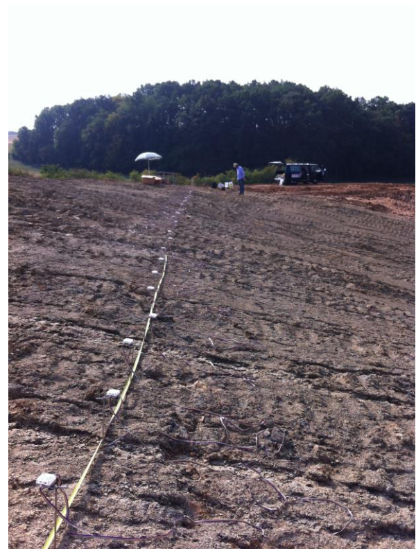
Figure 3: Measuring an ERT transect with the device of L-GM in the open clay pit near Buttenheim.
