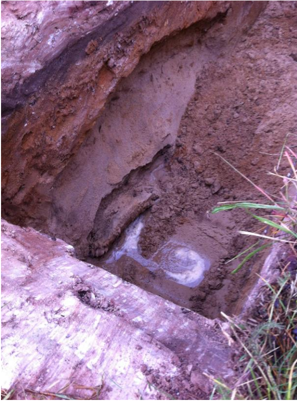
Figure 8: Ingress of water in one of the testing pits in Eltersdorf/Erlangen as indicator for the vadose-phreatic transition zone at the bottom of the test pit.
