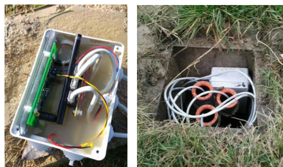
Figure 6: Prototype of the standalone underground sensors.
