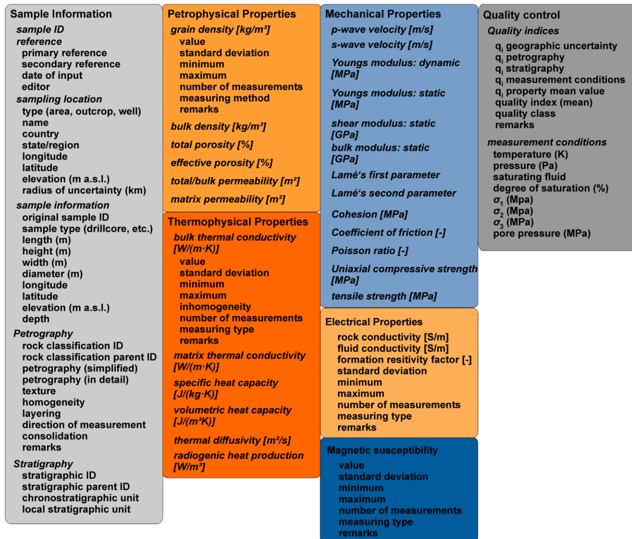
Figure 1: Schematic structure of the IMAGE rock property database illustrating the main three pillars: sample information, rock properties and quality control. Different input parameters (small font) are grouped according to the property they belong to (italics).
